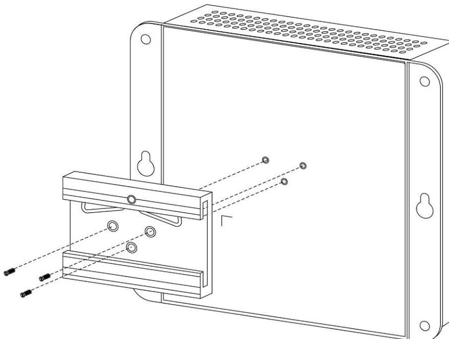
**Step 2:** Lightly insert the button of DIN-rail into the track.
