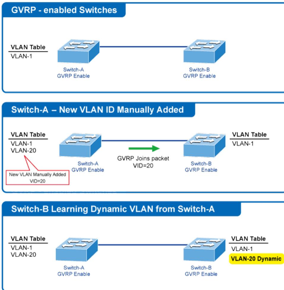
VLANs are **dynamically** configured based on **join messages** issued by host devices and propagated throughout the network. GVRP must be enabled to permit automatic VLAN registration, and to support VLANs which extend beyond the local switch.
