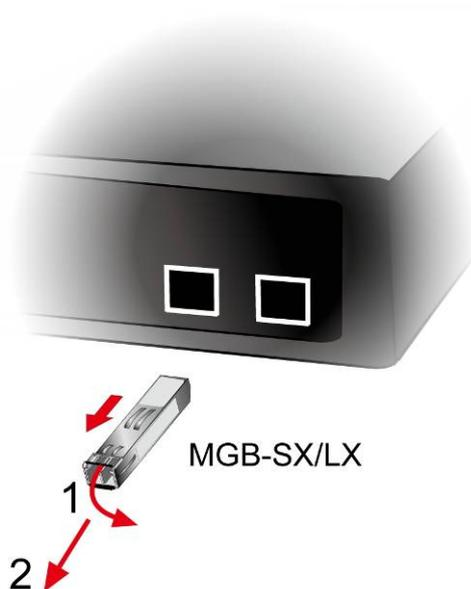
Figure 2-1-2f How to Pull Out the SFP Transceiver
