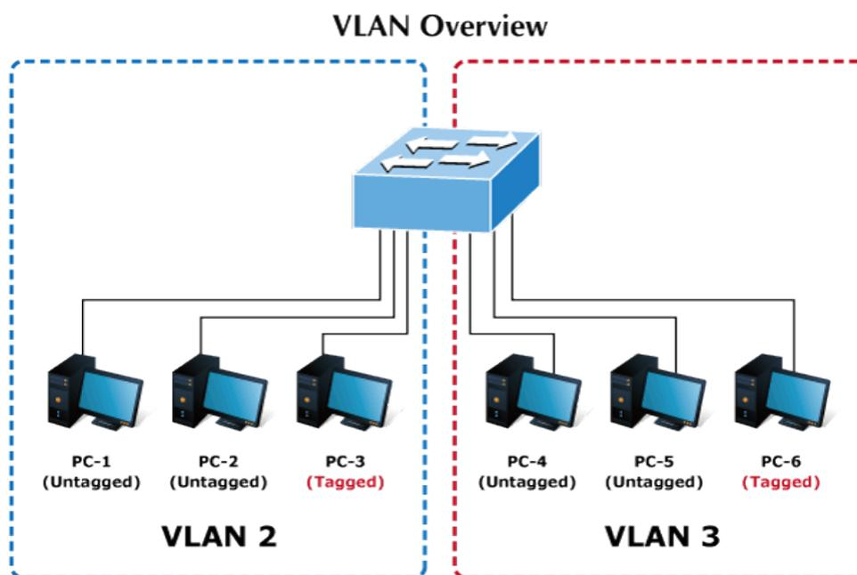
1. No matter what basis is used to uniquely identify end nodes and assign these nodes VLAN membership, packets cannot cross VLAN without a network device performing a routing function between the VLAN.
