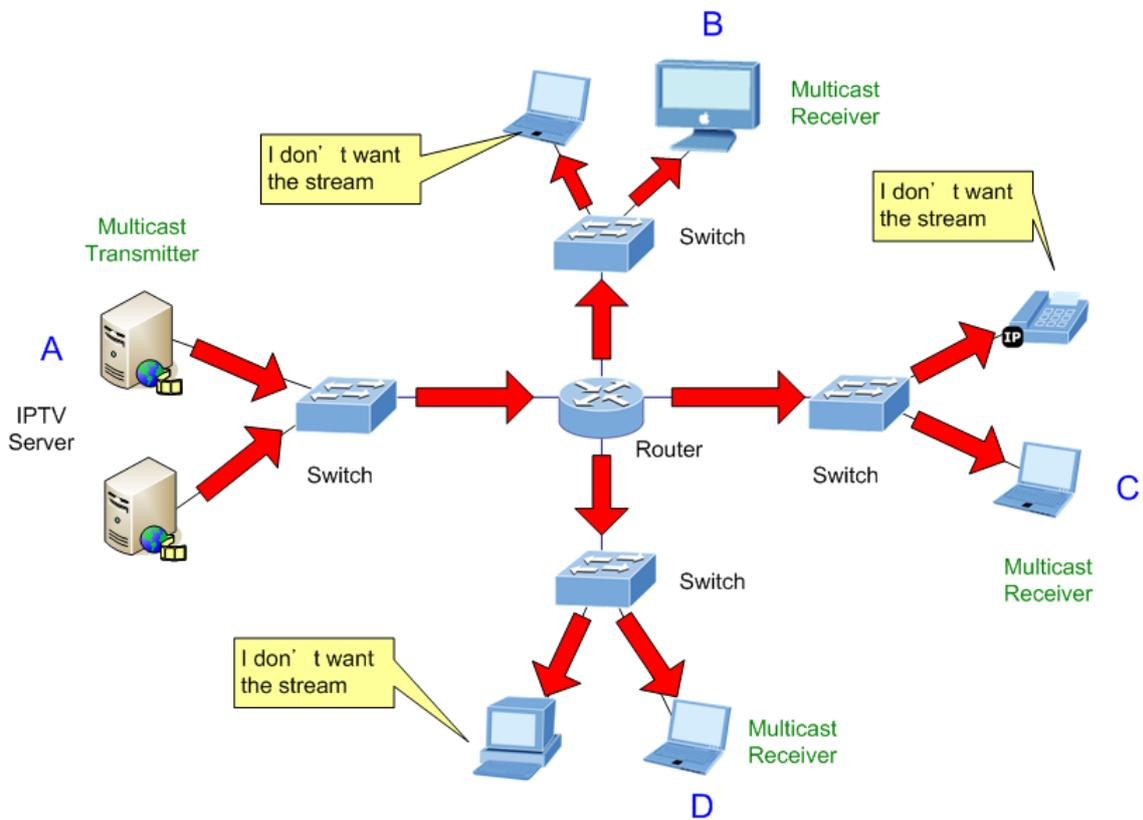
Figure 4-7-4 Multicast Flooding
