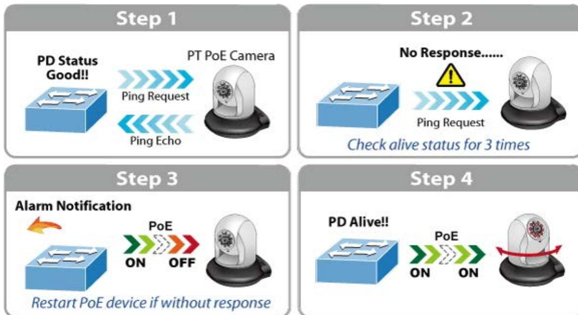
This page provides you with how to configure PD Alive Check. The screen in Figure 4-15-7 appears.
