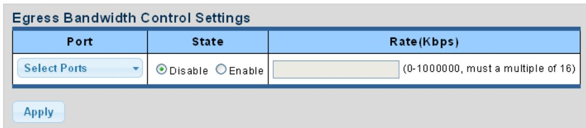
The screenshot shows the 'Egress Bandwidth Control Settings' page. It features a table with three columns: 'Port', 'State', and 'Rate(Kbps)'. The 'Port' column contains a dropdown menu labeled 'Select Ports'. The 'State' column has radio buttons for 'Disable' (selected) and 'Enable'. The 'Rate(Kbps)' column has a text input field with a placeholder '(0-1000000, must a multiple of 16)'. Below the table is an 'Apply' button.
