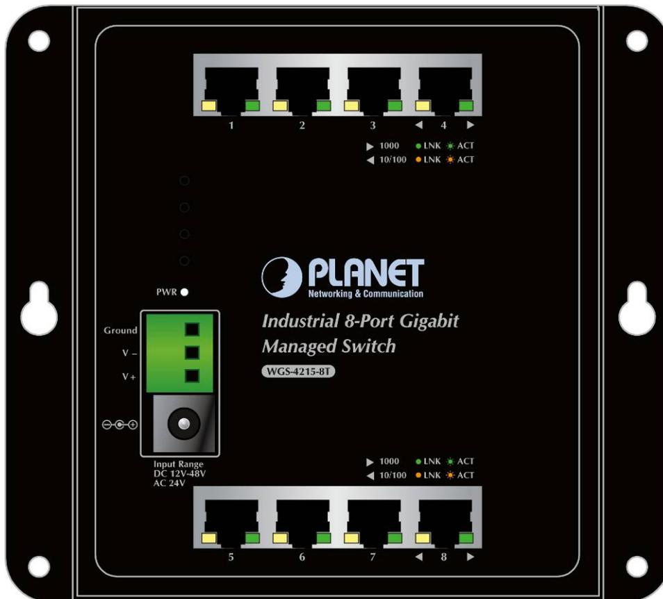
Figure 2-1-2b WGS-4215-8T LED Panel
