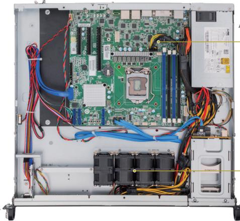
4 x 40mm Fix Fan, Dual Rotor
