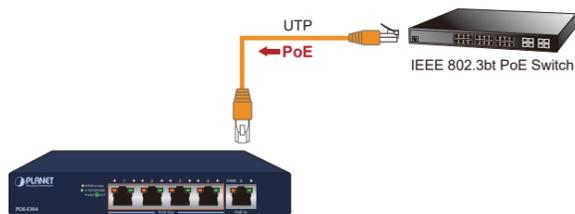
**Step 2:** The PSE delivers both Ethernet data and PoE power over UTP cable to the Gigabit PoE Extender.
