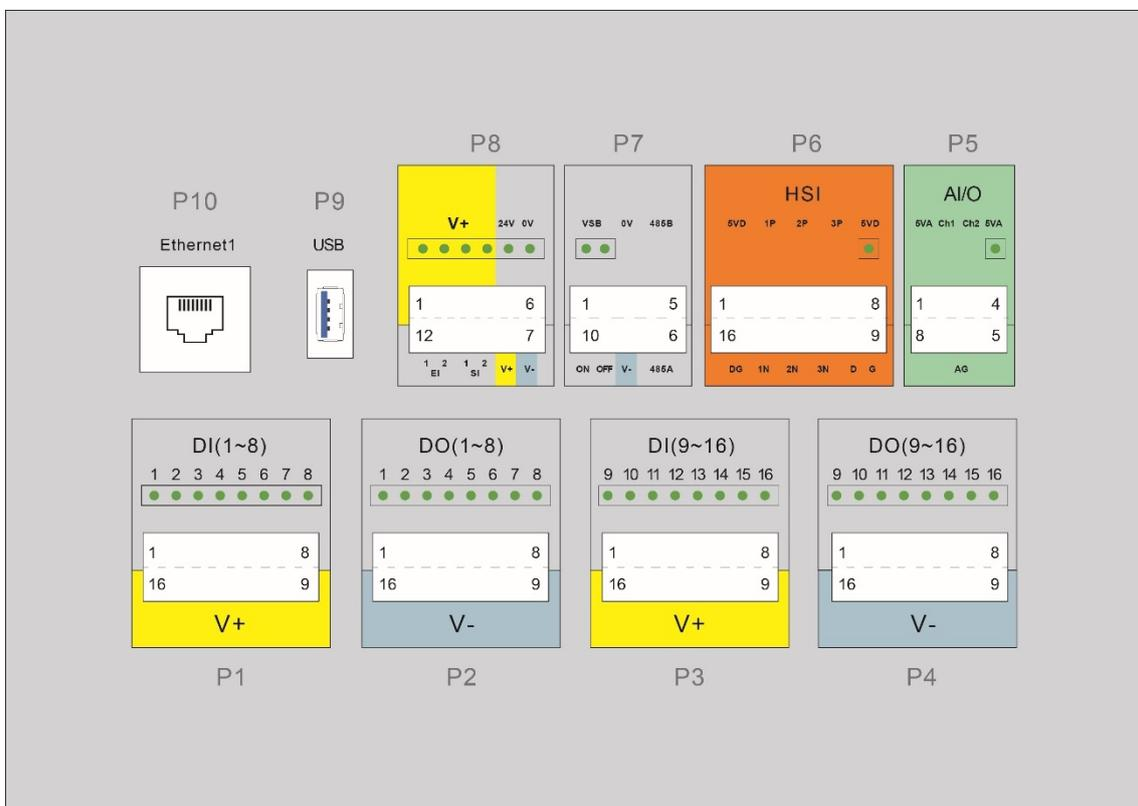
Figure 4-1 Front panel interface of the electrical cabinet
