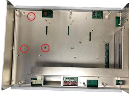
3. Attached the SATA cable to the HDD/SSD storage device. Slide the HDD/SSD storage device into the bracket and fix the storage device in place by fastening the 2 screws on both sides of the bracket .
