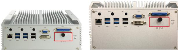
**Note:** Be sure to turn off the computer before installing or uninstalling the CF card if the OS is installed on the card.
