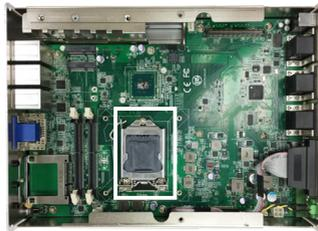
The processor socket comes with a lever to secure the processor. Please refer to the pictures step by step as below and note that the cover of the socket must always be installed during transportation to avoid damage to the socket.
