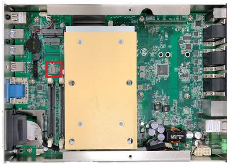
3. Slide the SIM card holder cover towards the OPEN edge and then lift the cover to open it.
