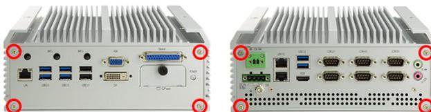
3. Carefully lift the top cover and then completely part the top cover from the computer.
