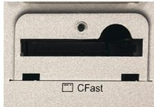
3. Position the CFAST card as directed by the graphic printed on the front panel. Insert the CFAST card all the way into the slot.
