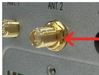
Mount the washer and the nut to the SMA connector. Tighten the nut.
