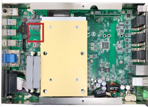
3. Prepare the Wi-Fi module kit. The module is a **M.2 E-Key** socket form factor, with two U.FL connectors, one is “MAIN”, and the other is “AUX”.
