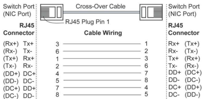
**NOTE** If the PD only supports PoE MDI mode (V+, V+, V-, V- for pins 1, 2, 3, 6), choose a cross-over Ethernet cable to connect the PD and the EDS switch. If the PD only supports PoE MDI-X mode (V-, V-, V+, V+ for pins 1, 2, 3, 6), choose a straight-through Ethernet cable between the PD and the EDS switch.
