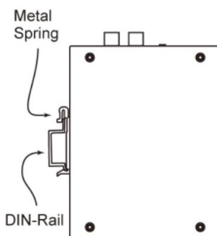
To remove the EDS from the DIN-rail, simply reverse Steps 1 and 2 above.
