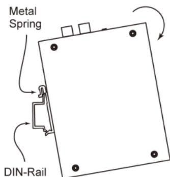
**STEP 2:** The DIN-Rail attachment unit will snap into place as shown below.
